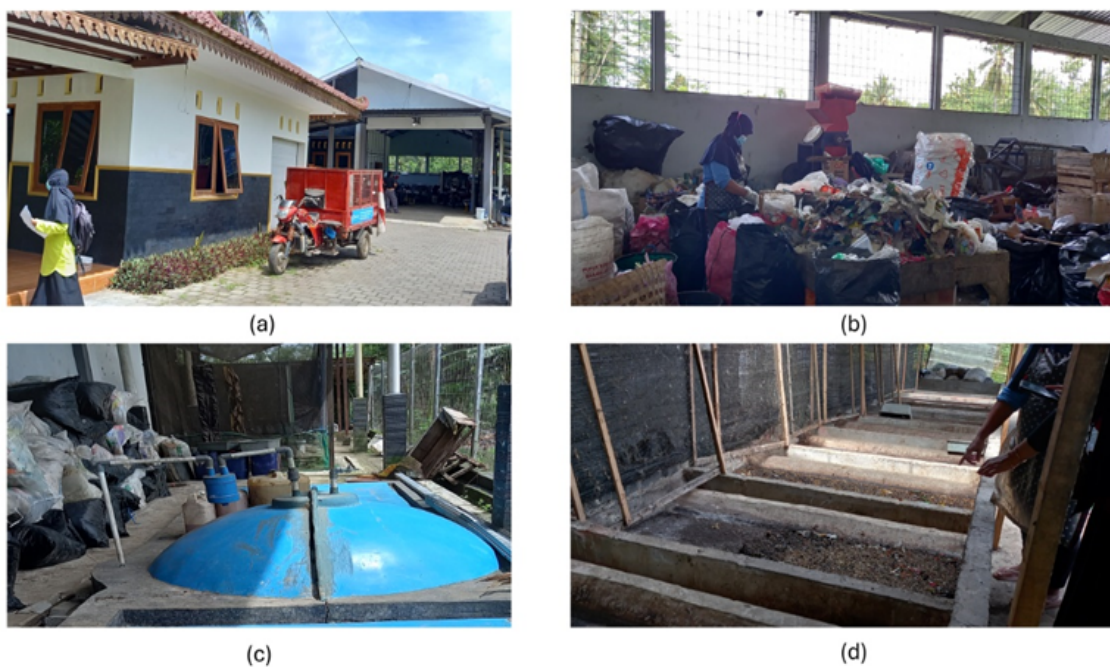
Figure 3. A typical TPS 3R building in the Borobudur sub-district consists of an employees' room in the front and a hangar in the back (a); household waste manual sorting in the TPS 3R hangar (b); an idled biodigester located in the TPS 3R backyard (c); and maggot cultivation feeding with food waste (d).
