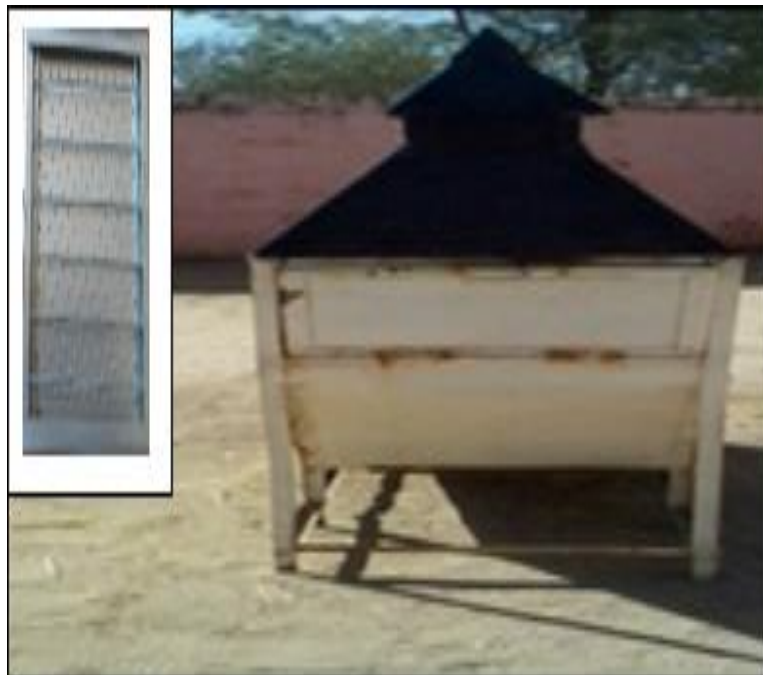
Figure 2. Drying chamber with drying tray
