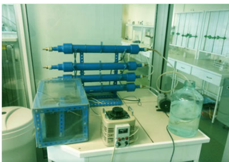
c) Disinfection of water using an ozonator unit of a small laboratory type
